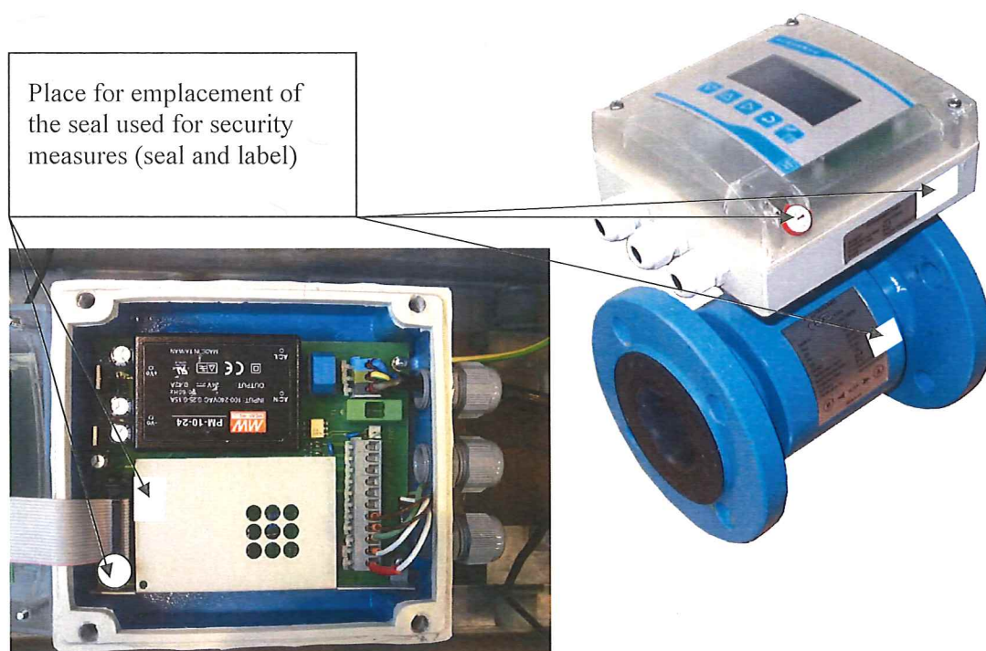
Picture No.3 Emplacement of seal used for security measures
